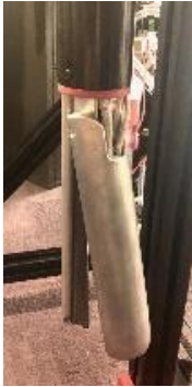
Fig. 4. Custom machined heating probe
